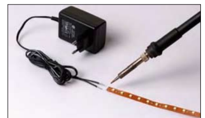
Solder leads to switching power supply indoor or outdoor type.
