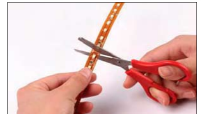
Cut to the desired length on the closest cut mark printed on the product.
