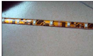
Reveal the LEDS by removing the cover tape.
